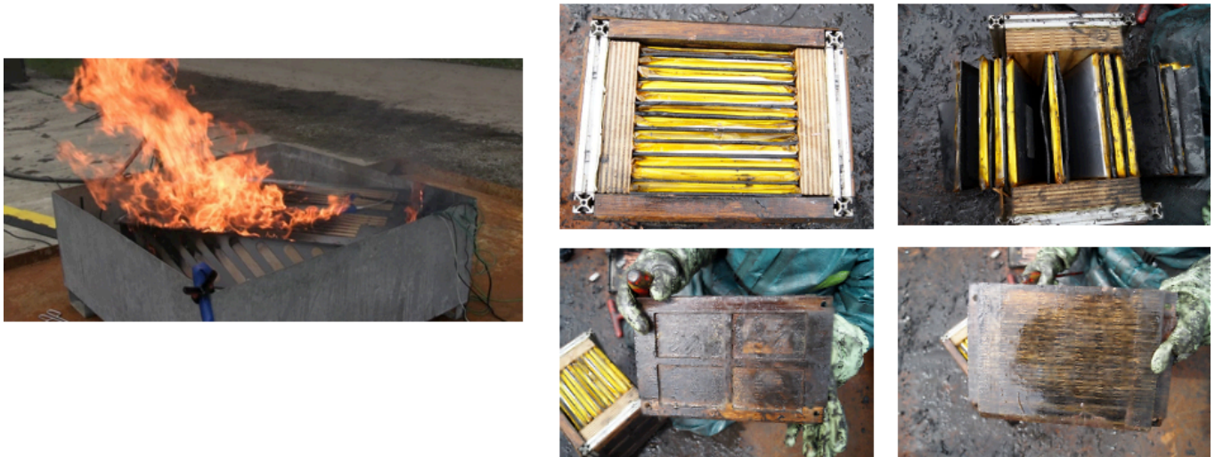
Figure 8: Abuse test on COBRA pack prototypes
