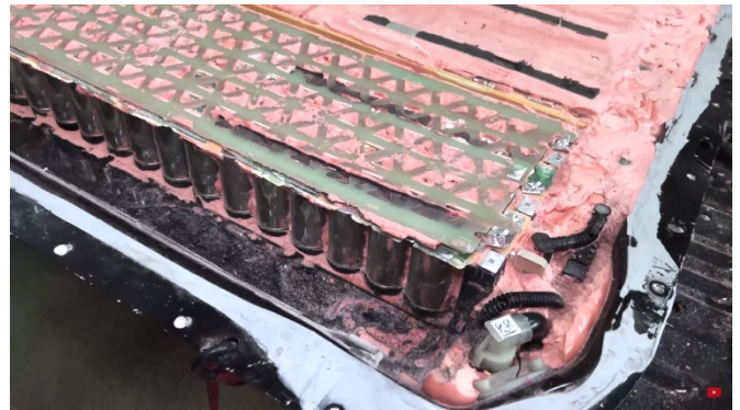
Figure 6: Tesla 4680 cell-to-pack design with PUR foam providing rigidity.
